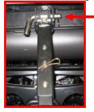
Pin in adjustable Link as shown here.
