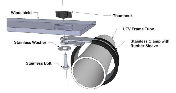
7. Now you can install the Bent Lexan Brace on the outside of the windshield along the top. This piece is optional to install if you are installing the windshield as a standalone item. It is designed to seal the cab when the windshield is mated with one of Mammoth Designs Cab Enclosures. Please see the diagram below for installation.
